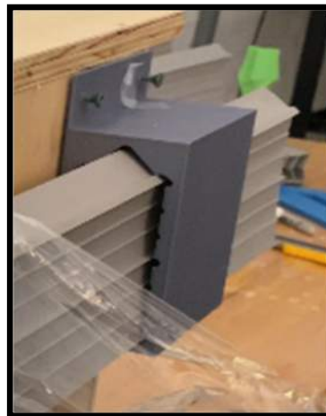
GASKET HOLDER for making corners
