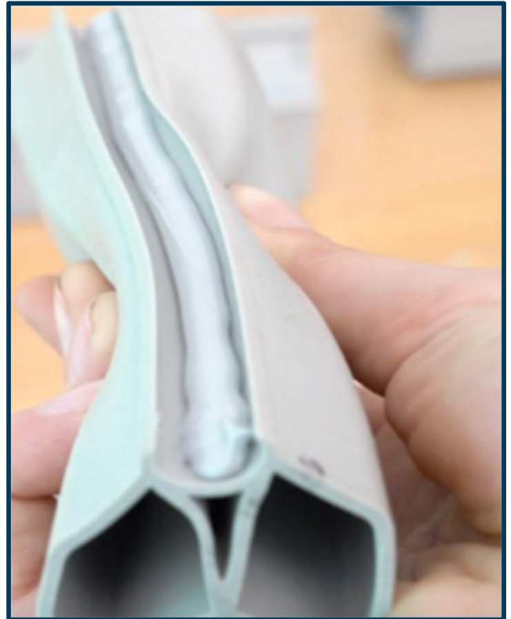
Place 1/8" bead of sealant continuous
